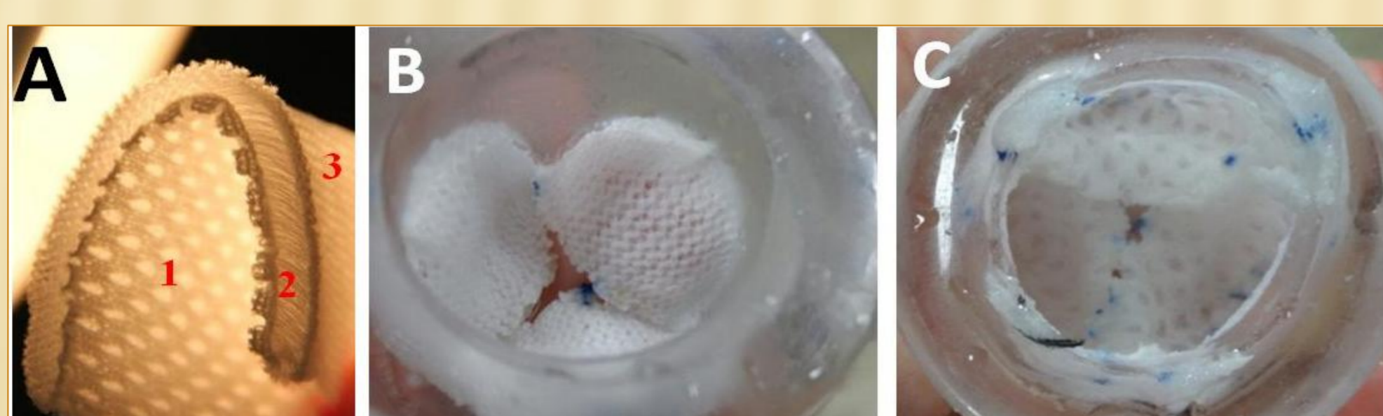
Figure 3. Three-dimensional weft-knitted spacer fabric made out of PET yarn originally made for sport-garment. 1,2,3 are three layers of fabric (A). The fabric was used to construct leaflets which provide a closer structural match to three layer architecture of leaflet than examples reported before (7). Ventricular (B) and aortic (C) sides of the valve construct.
