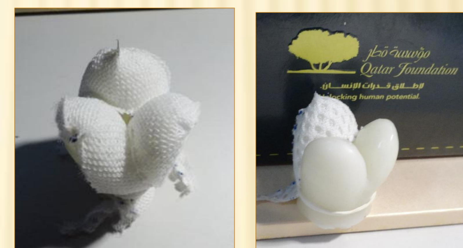
Figure 5. Prototypes of obtained 3D-knitted leaflet structure.
