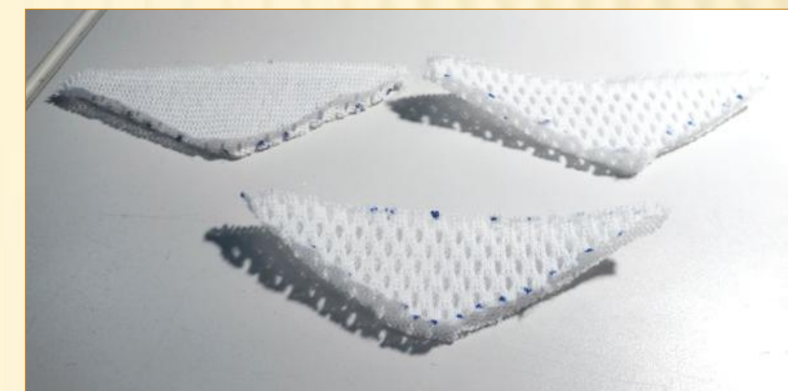
Figure 4. Structure of a 3D knitted fabric
